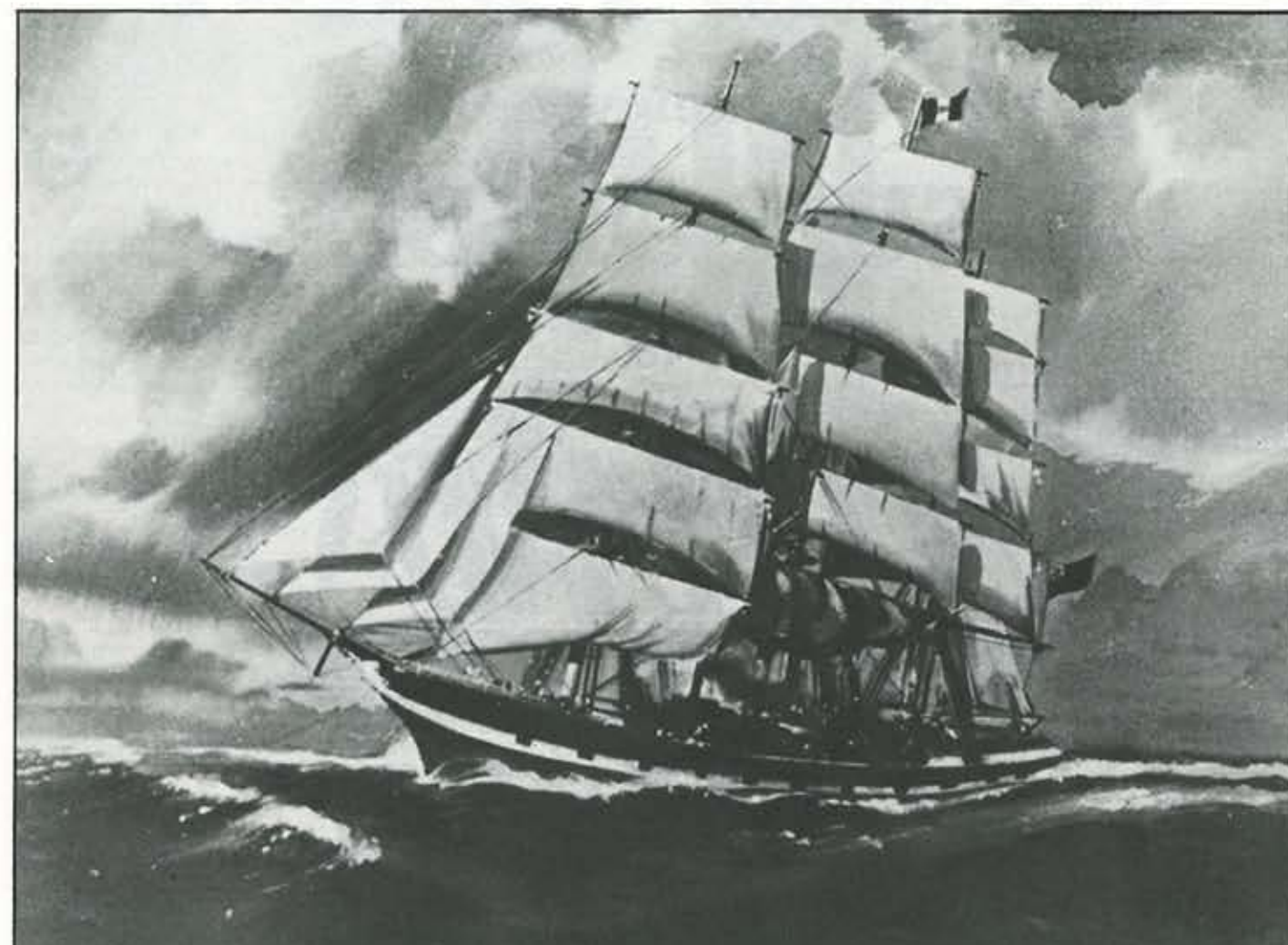
The full-rigged clipper Dunedin from a painting by Frank H. Mason. The funnel of the donkey engine driving the refrigeration compressors can be seen midships. The ship was lost in the neighbourhood of Cape Horn on a voyage back to Britain in 1890.
